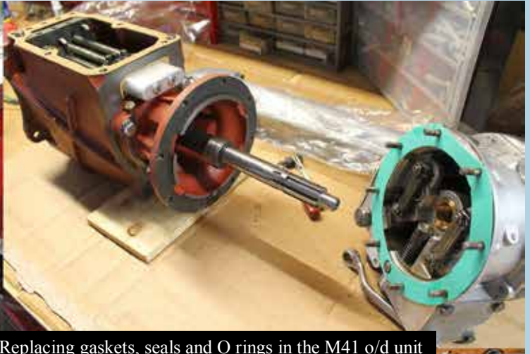
Replacing gaskets, seals and O rings in the M41 o/d unit
