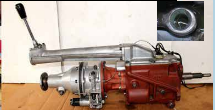
First time out of the car most probably. Cleaned up well needing a replacement gear stick bush which fixes up the vague gear change
