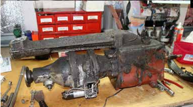
First time out of the car most probably. Cleaned up well needing a replacement gear stick bush which fixes up the vague gear change
